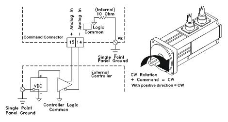
Figure 21: Analog Command, Differential Wiring Diagram
